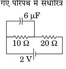
Find the charge on the capacitor as shown in the circuit.
